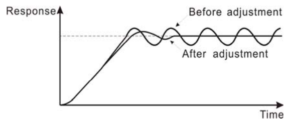
Figure 6.31 Reducing short-cycle oscillation diagram.
