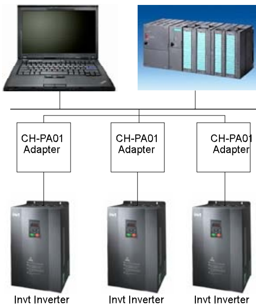
Figure 7.17 Profibus communication structure diagram
