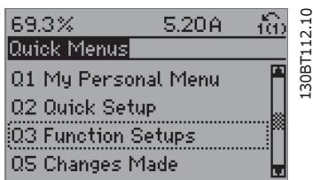
Illustration 1.9: Step 3: Use the up/down navigation keys to scroll down to Function Setups. Press [OK].
