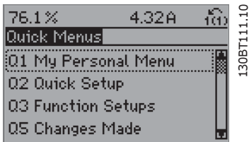
Illustration 8.2: Step 2: Press the [Quick Menu] button (Quick Menu choices appear).
