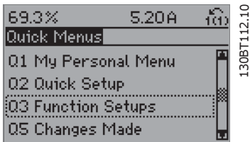
Illustration 8.3: Step 3: Use the up/down navigation keys to scroll down to Function Setups. Press [OK].
