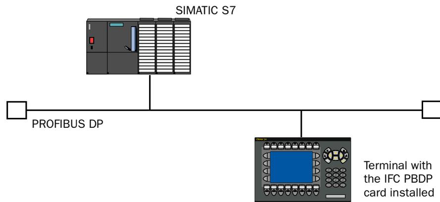
**Alternative 1: Current PLC project (HMI profile) for S7-315-2DP CPU**
