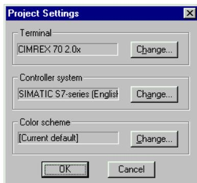
Press **Change...** under **Controller system** to get the choice list of available drivers. Choose **Brand name**, **Protocol** and **Model** and then press **OK**. Press **OK** again to confirm the project settings.
