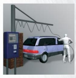
Operation control In coin-operated car washes the ZEN can change the program's operating time, depending on the number of coins inserted.
