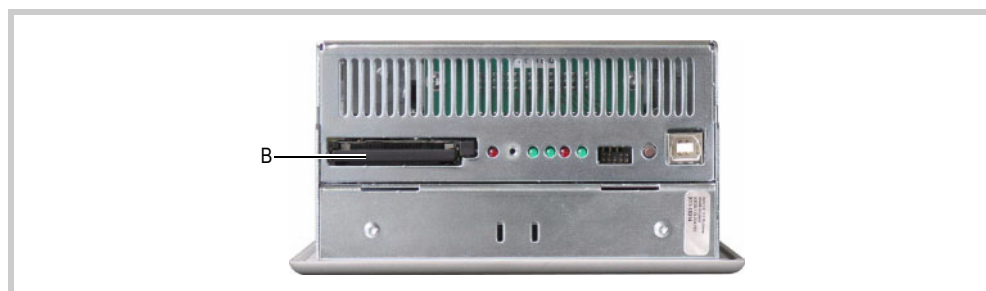
Fig. 43 Service side of the device (CF slot cover removed)
