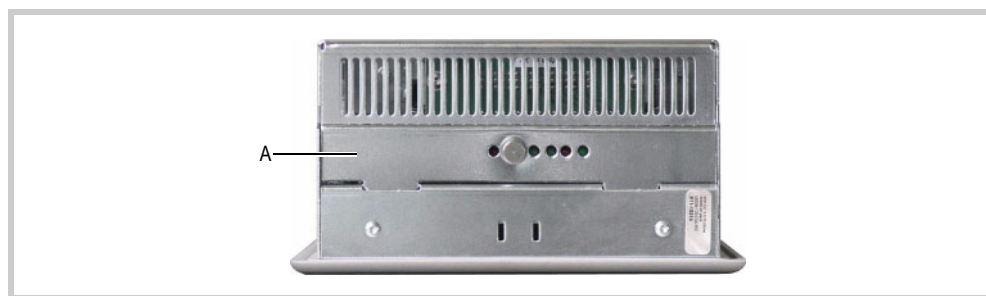
Fig. 42 Service side of the device (CF slot cover fitted)
