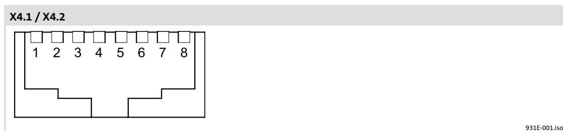
Fig. 7 Connection of CAN bus (X4.1, X4.2)
