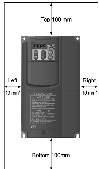
Figure 2.1 Mounting Direction and Required Clearances
