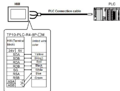
User-made cable is necessary, depending on the PLC.
