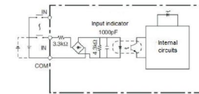
a) 2\*100 KHZ Internal circuit of high-speed input
