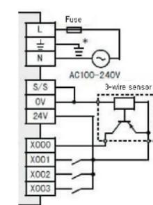
Wiring diagram of input terminal (Sinking/ sourcing)
